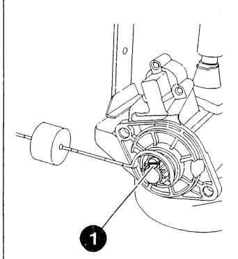
Checking armature braking torque
